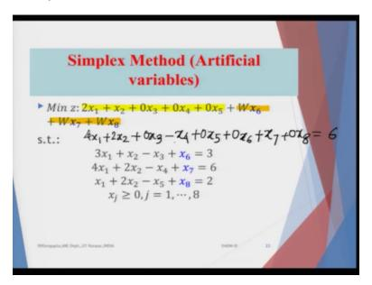
So the second row is this one. So this would be 4x1 plus 2x2 plus 0x3, because 3 was for the first constraint minus x4 which is there plus 0x5 plus 0x6 plus x7 plus 0x8 is equal to 6, so that becomes the second constraint and the values multiplied for each and every vector x is 4, 2, 0, minus 1, 0, 0, 1, 0 so this is the second constraint.
