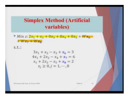
So let us check, because if I put x1, x2, x3, x4, and x5 all 0, technically x6 is equal to 3, x7 is equal to 6, x8 is equal to 2. So which maybe starting basic feasible solution based on which we can start our linear programming. So the parameter corresponding to the row which would
