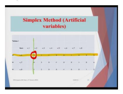
So we follow the same principle. (Like) trying to find out in the maximization and minimization case we take the maximum negative or the minimum positive based on which direction we want to move. And the pivot row and the pivot element would basically give me this. So I will basically mark the pivot row and I will mark the pivot element.
