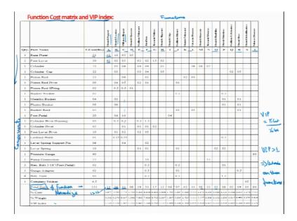
This is function cost matrix and value improvement potential, this was developed for the whole product. All the function are listed here functions from A to T in this line, and these are the components base plate 24 components are there, quantity is also here ok. These are the components here, I will put it here these are actually functions, these are components.
