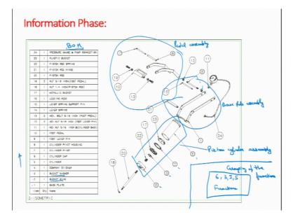
In information phase as I said, we develop the bill of materials, so this is bill of materials ok. Bill of materials is list of the materials with this is a phase search from the bottom number 1, 2, 3, 4, 5, 6 and so on. So, this list of material is developed and we have the very first component as base plates, secondary component is bucket ring, third component is company sticker, cylinder.
