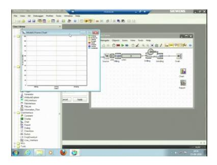
User interface means anything that the user could see after the process has run for one time. So, if this is I have a chart here and I try to just drag my process is here milling drilling so I am just trying to put the process is here ok. Now when I run my process it will show, you can see this chart.
