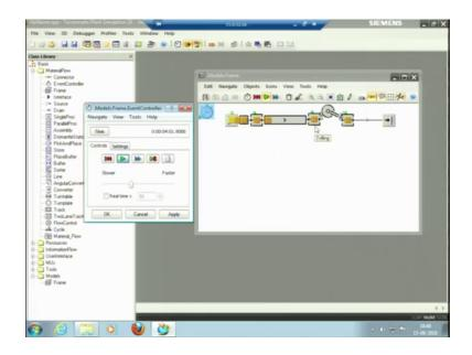
There is no material handling system. So, I like to put pick and place robot pick and place robot. I will these are the names if it is I will getting a little congested I can take this off using this command. So, delete this connector; now, I will connect using the pick and place robot.
