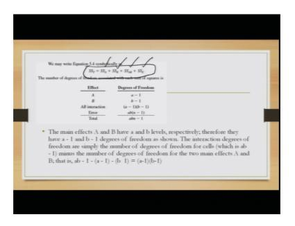
So, we can write the total equation as this, sum of the total squares would be for the rows, for the columns, for the combinations and for the error part. So, now, I have given is divided into two parts now pause here.
