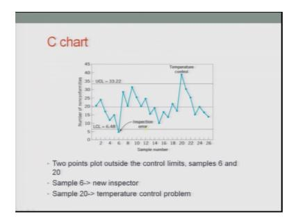
So, when we plot it two points plot outside the control limits, which are basically sample 6 and sample 20. So, say for example, so hypothetical excuses or reasons not I would not use the word excuses the reasons for which the non conformity for those set of values came out may be that the broker on the new machine was a new operator. And obviously,
