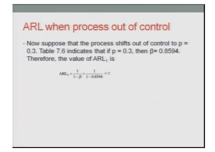
Now, suppose that the process shifts out of control to p value of 0.3, then again doing the calculation the average run length basically comes out to be about 7. Now, we will consider the control charts for average number of nonconforming conformities.
