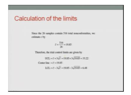
So, hence if I want to find out C s bar which is the best proxy of c that value comes out to be 19.85 and corresponding values of upper control and the lower control limit basically comes out to be about 33.22 and 6.48.
