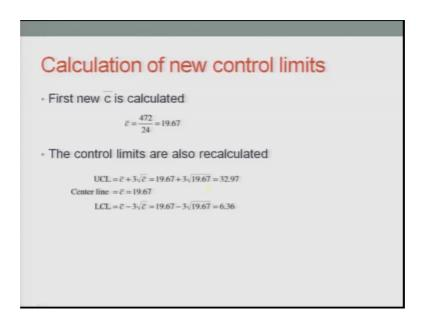
So, the new calculations first calculate the new c star or the c hat and the value comes out to be 19.67. Once you find out the value of 19.67, the control charts are drawn which means the upper control limit the lower control limit you find out basically UCL and LCL which would be c or c bar plus minus 3 of basically square root of c or c bar. And
