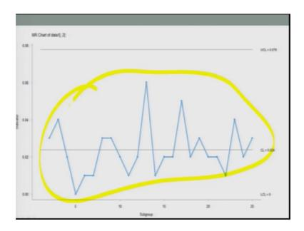
So, the ranges are given in this way the central line is 0.024 based on the calculation of the central line the upper control values is given by 0.078 and the lower control value is given by 0. So, obviously, you have the overall charts for each and every moving range values are like this. So, you know to basically need to comment about intelligently about the normality.
