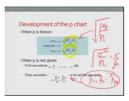
So, when p is known the proportions of defects or non defects are known the upper control limit and the lower control limits are given by upper control limit is given by p plus this three value is again coming from the overall variability of plus minus three sigma. So, this is three in the upper control limit, three in the lower control limit are those facts are taken in to consideration that I am trying to find out plus minus 3 sigma accordingly.
