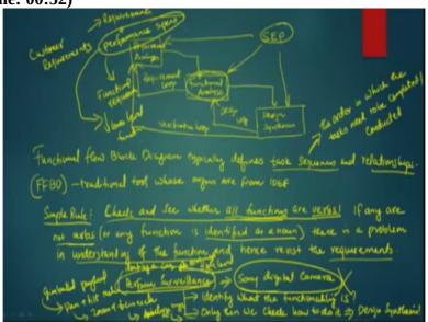
Systems engineering process loop had three things, the first loop is called as the requirement loop or the requirement, instead of the loop, we will call it as analysis. From here, we go to the next 1 which is called as functional analysis and then we have what we call as a design synthesis. So the requirement analysis gives rise to functional analysis, in this process you go back and check your requirement analysis and this is called as the requirement loop, okay.
