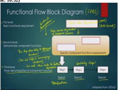
The functional flow block diagram has actually three, we can have multiple levels out of it also, typically you find it in three levels, the first level here, then the second level here and then the third level here, okay. So the first level is the basic functional requirement is what gets stated here. So you state the requirement here, the basic functional requirements gets stated there in the box, okay.
