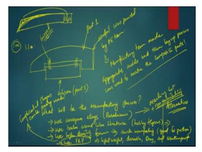
So the side piece if you take the left side piece it was fabricated something like this. It was created this and then. If you assume this is the wing piece this much of the wing was -- this much was built as first part of the wing and the aileron this was part two and this was part one. So the manufacturing process made this in two separate parts and then they were these were hinges they were hinged onto the general structure of the weight.
