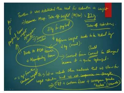
So then the further it was established the need for reduction in weigh because why was it is necessary because maximum take-off weight or MTOW was fixed somewhere at 22 kilograms it could not do better than this because of the take-off restrictions, okay. This was the take-off restrictions. So once this was there we said okay fine no matter what happens we have to reserve somewhere close to 3 kg for payload. Okay.
