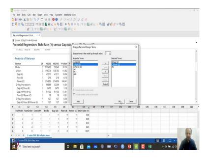
So, in this case in terms of terms what we will do is that, we will go to second order up to second order terms over here. So, here also AB is not significant we can remove this one. AC is significant. So, B can also be removed because B is not making significant impact on the overall CTQ or the response variability it is not impacting, we can remove this one.
