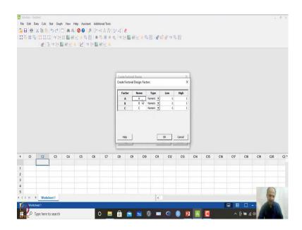
And then in factors we can assign the names over here, we can write names over here. And we can write the levels also. So, it is already coded, so I am using coded variables. All are numeric values that we are assuming over here and all are continuous variable that is why this numeric variable we are assuming. So, this is already done and that factor already is mentioned.
