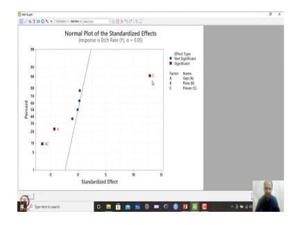
And also, this is prominent in the normal plot what you are seeing over here. So, in normal plot also you see that A is having a negative impact on the Etch rate and AC is having a negative impact, but C is having a positive impact on the Etch rate like that ok.
