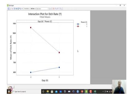
So, if we click ok over here then you will find that AC interaction is shown over here. So, interaction plot is given, and in this case, you can understand that to maximize the CTQ, let us see etch rate over here. This is the point I have to look it over here and this is corresponding to gap minus 1. So, A should be in negative level and C should be in positive levels.
