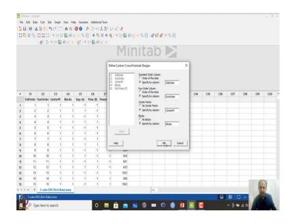
So, these this is the low level. So, this worksheet we can say that this is what, data is coded over here. So, I will place ok and design over here. So, specify the columns by. So, this is the standard order where it is mentioned. So, I have taken the standard order over here. Then run order what I will mention is that this is the run order over here.
