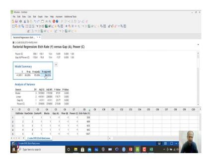
And R square predicted value is around 93 percent what we are seeing over here. So, I can copy this from here and we can paste it over here, and then enhance this one, so that it is visible to you. So, this is 93.02 which is which is very good basically, which is very good over here. So, now I have eliminated some of the factors which is unnecessary over here which is B over here.
