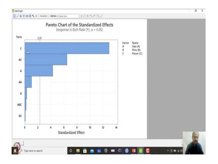
What we can do is that, we can click ok and try to see the effect plots over here and what happens let us try to see ok. So, when I have made the plot over here in the effect plots what we see is that, here A, C, and AC these are the factors what you can see over here. A, C and AC is primarily predominantly is having effects which is significant effects over here.
