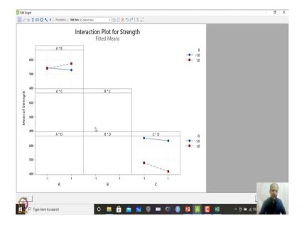
So, in this case we will use factorial plots over here. So, ABCDE and only a model terms that we will use, and in this case we will click ok. And then we will have this interaction plots we will have this interaction plots which will define what should be the level of A and B. We want to maximize the strength over here.
