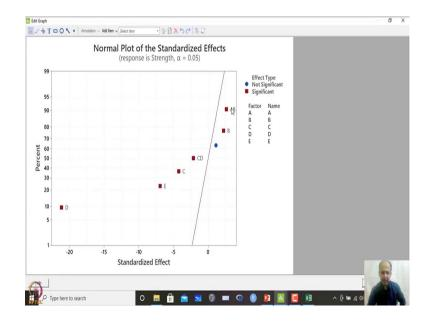
So, this is the this is the model, and also what is visible in the normal plot also we will find. So, AB and B have a positive impact, and C, E, CD, and D have a negative effect. So, AB and CD is important and other factors also levels. Only thing is that A will be defined which level based on AB interaction we will define what should be the level of A, and other things we can see it like CD interactions.
