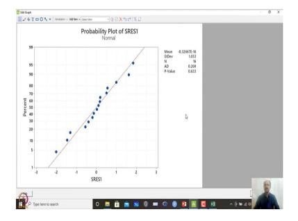
So, last column will be basic standard residual plots over here. So, I can use the residual, and I can just check Anderson Darling test and what we are observing over here in Anderson Darling test, is that the P value is more than 0.05. So, in this case normal normality assumptions is not validated at least.
