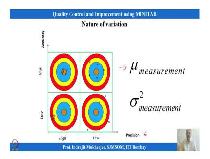
So, this is what we have seen earlier also in the diagrams for when we are talking about accuracy and precision. So, when we are talking about precision, we are talking about sigma aspects of this. When we are talking about accuracy, we are talking about the mean of this over here measuremental system mean whether it is shifting like that.
