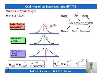
So, all this to ensure that the instrument is correct, we need to understand one important topic which is known as Measurement System Analysis. So, whatever  $C_{pk}$  values or variability analysis, ANOVA analysis that we are doing, we are assuming that the overall variability is correct and overall variability, total variability that we are measuring is correct.
