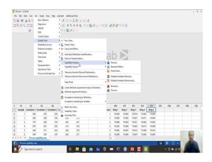
So, this data set is already I have created. So, a Minitab file I am opening. This is the observations of one dataset, this is the other observation which we will analyze now sample pistons – ring 1 to ring 5; 5 sub groups and these are the observations over here.
