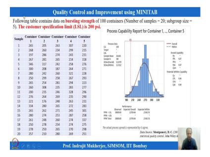
And, we have an example over here that is container over here. So, here in this example what you see is that 5 container subgroup size is 5, but LSL is only given 200 over here. So we have 20 samples with 5 observation. So, total 100 observations we are having 5 subgroup size. So, total 100 observation and lower specification limit is given as 200 psi.
