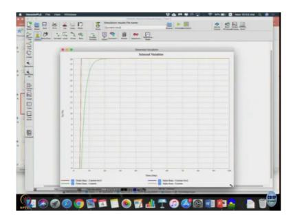
The order rate and sales rate are exactly the same, I just overlapped the previous simulation run along with this one, to get the exact same behaviour for the order rate and sales rate so; that means, addition of the sales rate actually did not affect my order rate.
