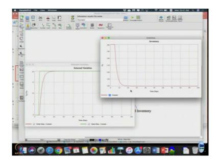
We have already seen this when we were discussing negative feedback system in phase of constant exogenous output your steady system reaches equilibrium, but at a value different from the desired value. And the amount will be equal to the time to adjust inventory multiplied by steady state value of the sales rate in this particular case.
