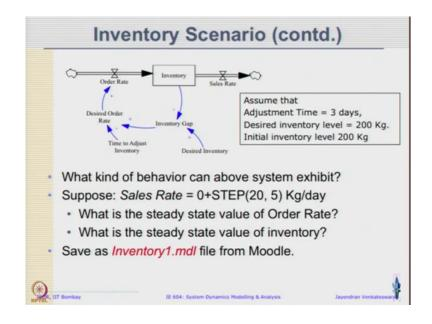
So, let us open Vensim and start modeling this; to get the values you can assume the following. Adjustment time is 3 days, you can take the simulation length as 100 and the simulation length as time step as 1 and the time units as base; go ahead and build this model.
