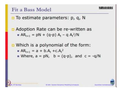
So, not a fit a bass model to estimate these parameters p, q and N, we need to estimate and we wrote it, we rewrote the equations adoption rate and we got this polynomial of this particular form.
