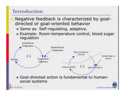
We have seen the negative feedback is characterized by goal-directed or goal-oriented behavior. Common similar terminologies includes self-regulating or a adaptive terminologies end up using. Most of the control systems models where there is feedback involved falls under this category where you are looking at current state versus actual I mean desired state, and then start taking gap between with them and try to control the system.
