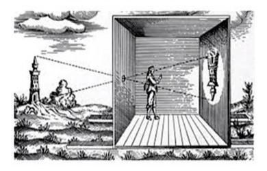
So here this is a pictorial representation of camera obscura, which suggests about its functioning.
