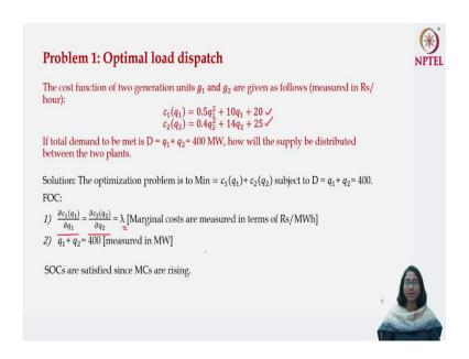
Let us have a quick look at one of the simple problems on optimal load dispatch. The cost function of two generating units  $g_1$  and  $g_2$  are given as follows. The costs are measured in terms of rupees per hour. The cost function is  $c_1(q_1)$  for the first generating unit and  $c_2(q_2)$  for the second-generation unit. For the first-generation unit, the cost function is given as  $0.5 q_1^2 + 10 q_1 + 20$ . This has the quadratic form.
