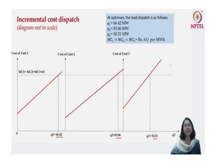
The diagram shows the production by the first unit which is 66.42, the production by the second unit and the production by the third unit and marginal costs is equalized at 63. The most efficient plant is unit 2 which is producing the most, followed by the next efficient unit which is the first unit and the third unit produces the least amount of output.
