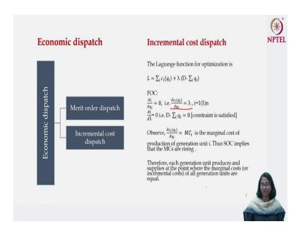
For the optimization problem let us set up the Lagrange function in the following manner. So, L is the Lagrange under consideration, we need to minimize this total cost therefore, the Lagrange is written as  $L = \sum_i c_i(q_i) + \lambda (D - \sum_i q_i)$ . If  $D - \sum_i q_i = 0$  that implies
