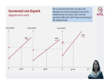
The diagram gives the general understanding of what is going on. It shows the marginal cost of the first generating unit, the marginal cost curve for the second generating unit and the marginal cost curve for the third generating unit. The intercept is lowest for the second generating unit followed by first and third generating unit.
