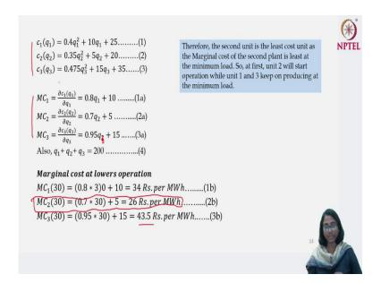
Let us have a look at the marginal costs first. Taking the derivative of these three-cost functions, we get the marginal cost functions. By taking the derivative of  $c_1$  with respect to  $q_1$ , the taking the derivative of  $c_2$  with respect to  $q_2$  and the derivative of  $c_3$  with respect to  $q_3$  give us the marginal cost functions  $MC_1$ ,  $MC_2$  and  $MC_3$ .
