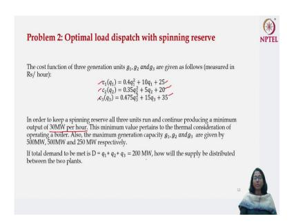
The optimal load dispatch problem becomes a little bit complicated if you think about the spinning reserve. It is not only the equalization of marginal cost but also having to ensure that all the plants under consideration that are supposed to run, have to run on a minimum load.
