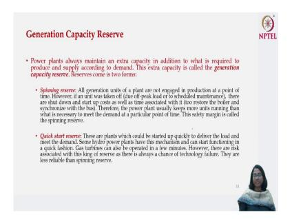
Another concept is called generation capacity reserve which follows the concept of the load dispatch. The power plants always maintain an extra capacity in addition to what is required to produce and supply according to demand. If my demand is 400 megaWatt, then I would try to
