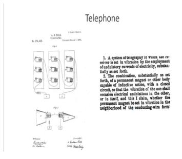
Telephone again and here is the claim of the telephone. A system of telegraphy in which the receiver is set in vibration by the employment of undulatory currents of electricity, substantially as set forth. So, for lay a person a telephone is how it looks to him, but for the purposes of patenting you need to textualise the invention in a determined manner in such a way that you can convey what is been invented and what is been protected.
