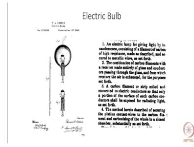
Now to give you an overview of how this looks. The electric bulb we saw the patent, and there was a description a drawing in the patent. But the way in which the electric bulb is described in a claim is as an electric lamp for giving light by incandescence, consisting of a filament of carbon of high resistance made as described and secured by metallic wires, as set forth.
