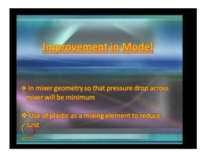
Next is, improvement in the model, mixer geometry should be improve, so that the pressure drop across the mixer will be minimum, we can use a plastic as a mixing element to reduce a cost of model. Thank you.
