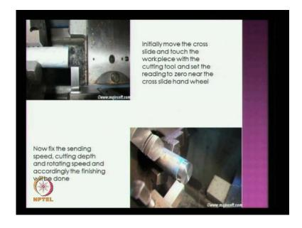
And then, initially move the cross slide and touch the workpiece with the cutting tool and set the reading to zero near the cross slide hand wheel. Now, fix the sending speed, cutting depth, and the rotating speed accordingly the finishing will be done.
