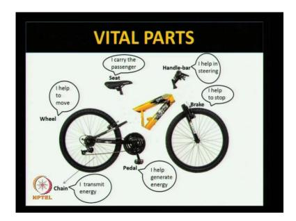
The Bicycle skeleton has several important parts, the seat carries the passenger, the handle bar controls the direction, the brake reduces the speed, the pedal is where the foot rests and generates energy by rotation. The chain transmits this energy to the wheel which manifest itself in forward motion.
