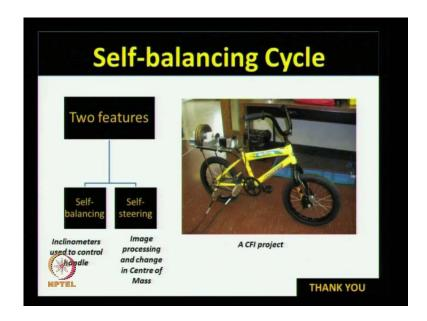
A group of students from our very own institute, had improved upon the existing design of the Bicycle, by building, a self balancing cycle, this prototype could self balanced using inclinometers, and also self steer using image processing, and self balancing tool. Bicycle is a very useful and highly efficient engineering product. Hence, it is no one that, so many bicycle thefts a reported in the our institute. Thank you.
