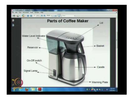
These are some of important parts of a coffee maker. Now coming to the process, initially the brown coffee beans are placed in the shower head, and water is poured in the reservoir.
