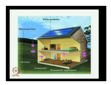
A typical photo voltaic system includes an array of solar panels, an inverter, controller, and then electronic box.
