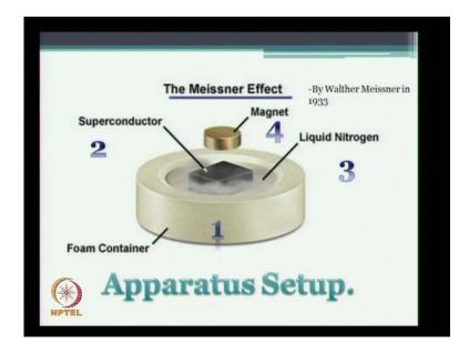
And we require a foam container a superconductor some amount of liquid nitrogen, and magnet. First, we take a foam container, and then we place a superconductor at the center of it, and then very slowly and very carefully, we pour the liquid nitrogen in the container, and by wearing proper glasses and gloves, then we try to place the magnet over the superconductor using tongs, and we see, that the magnet gets levitated in the air, and that is the magnetic levitation.
