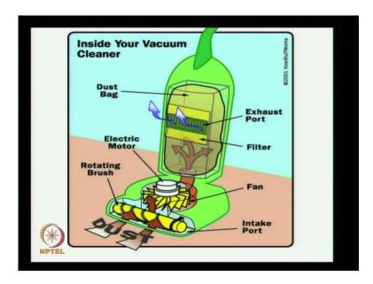
The vacuum cleaner consists of the following parts; Intake Port, Fan, Rotating Brush, Electric Motor, Dust Bag, Filter, and then Exhaust Port.
