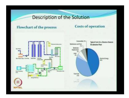
A flow chart of the process is shown in the slide along with the cost of operation, around 44 percent of the total cost is used up in supplying electricity to this process. Hence, critics believe that, this will result in an increase in the green house emissions. However, the company has assured that this can be reduced by purchasing carbon credits and also
