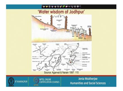
So, this is the snapshot of the 'Water wisdom of Jodhpur'. So, you can see and integrated you know an integrated water system. So, how you know the canals, the barns, the wells, and the tanks, they are all you know embedded and integrated as a single system for you know for irrigation purpose in Jodhpur and, also for other purposes including the supply of drinking water and all that.
