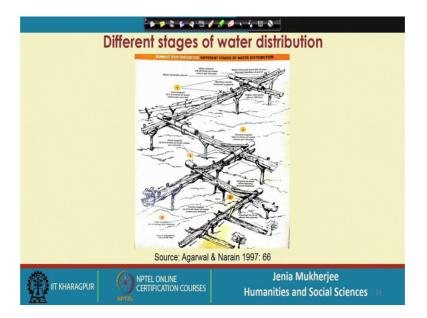
So, this is the illustration reflecting on the different stages of water distribution through you know bamboo pipes and for each of the stages so, this is stage 1, stage 2, stage 3. So, at each stage find you know difference in the amount of water entering through this bamboo per minute so, an extremely sophisticated system ok. And finally, stage 4, stage 5 so, stage 5 by 10 to 20 drops of water enter to this bamboo per minute and finally, you know before got it got transmitted to the plans.
