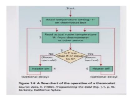
Now here you can see flowchart of how the thermostat actually functions. So at the top you can see that the thermostat needs to start and the first step that it will take is actually it will read at the thermostat box. What is the temperature that is being registered at the thermostat box? The second thing is it then reads the actual room temperature wherever the thermostat is actually placed okay.
