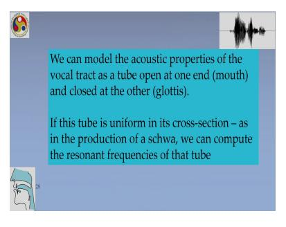
We can also model the acoustic properties of the vocal tract as a tube open at one end and closed at the other. So if this tube is uniform in its cross-section as in the production of a schwa, we can compute resonant frequencies.
