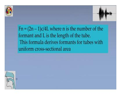
And there is a formula where you have, n is a number of the formant and, L is the length of the tube. And this formula derives formants for tubes with uniform cross-sectional area. So this is how we get the formant values.
