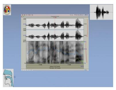
As you can see here, the first part of this diagram is that of a waveform. And this is a spectrogram, where you see the pitch is shown with the blue line; the intensity with a yellow line.
