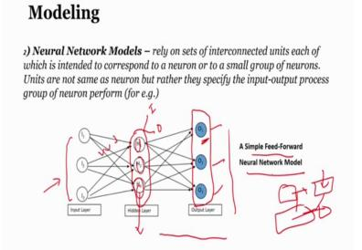
Now, this type of neural network structure that I am showing you is A Simple Feed-Forward network, what happens here is there are 3 units 1 1 1 2 and 3 3 which inputs which have been taken and these inputs are then compared or then processed through H 1 H 2 H 3 3 different brain networks or neuronal networks.
