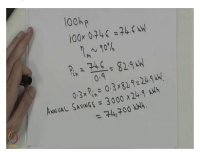
So, let us start by looking at if you are talking of 100 horsepower that will be 100 you can is 0.746 that is 74.6 kW is the full load rating of the motor, the efficiency of the motor is 90%. So, the input power that is required at full load is 74.6 by 0.9 which comes out to be, this is you can calculate this as 82.9 kW.
