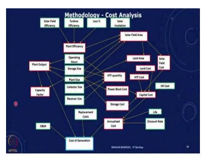
For instance, this is the cost of generation from a solar thermal power plant and you can see that when you look at it we are talking about the field, the efficiency, technical parameters, the plant output which will depend on the insulation solar field cause, capital cost, storage cost, annualized cost, replacement cost, discount rate.
