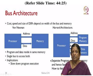
So coming to the bus architecture it depends on the cost, speed and size of DSP process basically width of the bus and memory. So, we have 2, architecture a lot of for normal CPUs use Von Neuman architecture whereas DSP processor use the Harvard architecture. So, in this case both address and data bus as you will be seeing that program and data reside in the same memory and single bus to access both your address as well as data, so which is going to slow down the program execution.
