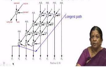
So we will see the architecture how does it look like so, most of the DSP processor use a Braun multiplier, you can see that  $4 \times 4$  Braun multiplier how it is represented. So, this is your full carry. So, I have an operand and previous carry n is going to be input of this and the second operand is coming from the side and the result is going to be sum and then carry out is going to be generated from full adder is shown in this way. So, we say that I need because we have taken m = n = 4.
