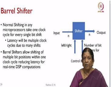
So, how we can accommodate the shifting? So, we know that sequential shifting is going to cost us n clock cycles if we need n bit shift. So we have a barrel shifter that is normal shifting any microprocessor that is what, what it says 1 clock cycle for every single bit shift. So what the latency will be multiple clock cycles due to many shifts. Whereas the parallel shift is allow shifting of multiple bit positions within 1 clock cycle, reducing the latency for a real time DSP computation.
