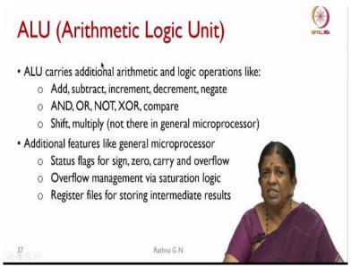
So, this is arithmetic logic unit apart from addition it has to take care of are the increment decrement negate or other operations and then shift multiply and additional features in the like other processes we should have a status flags for sign, zero, or carry or overflow. And then overflow management via saturation logic can be incorporated and registered files for storing the intermediate results.
