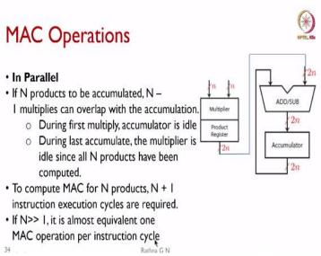
So, coming to MAC operations, we said in parallel what it is going to happen, so, what are the things we need it. So, if N products to be accumulated, we know that we need N minus 1 multiplies can overlap with the accumulation basically, that is during the first multiply accumulator is going to be idling. In the next clock onwards, we can do the thing parallely and the last clock cycle, because 1 value is left out to be added. So, this will be adding the last product.
