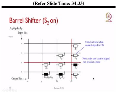
So, as an example, how the switching is going to be done is shown in this. So, what is the result I want  $A_2A_3A_3A_3$  on the my B zeros. So, you will be seeing that  $S_2$  switches closed wherever you have seen the  $S_2$  switch you have it is marked highlighted here. So, these are the ones which is going to these lines are going to be connected. So, when you connect this one what happens, so, you will be seeing this red line correct.
