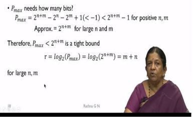
So we will see that how  $P_{max}$  can be represented. So, we have represented this and what the term is going to say is this terms can be represented as minus 1 that is it should be less than or equal to  $2^{n+m} - 1$  for positive n and m. And approximately if n and n m are very large, we can approximate this  $P_{max}$  to  $2^{n+m}$ . So therefore, we say that the maximum number of bits required to represent the product is less than  $2^{n+m}$ .
