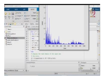
So; the next one is you will be seeing the error that is time versus mean square error. So you are seeing initially which was high and then which it has got considerably reduced. So this is how you would be doing the noise cancellation so using adaptive filter so the next one what we will see is after the noise cancellation.
