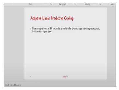
How your linear predictive coding is going to work, that is error signal from the linear predictive system basically what we have it so, that is system has a much smaller dynamic range in the
