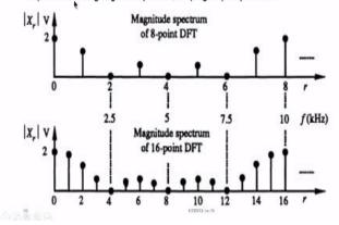
So, then know to check the thing how to calculate all though we have done it in the last class, we will see how to plot our magnitude spectra with an example. So, the example is x(n) = 0.5V for  $0 \le n \le 3$  and x(n) = 0 in other places, then compute the DFT for lengths of 8 and then 16 and plot the resulting magnitude spectrum sampling frequency in 10 kilohertz.
