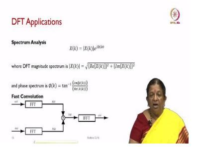
So, now what are the applications of DFT so, the first one as I told in the previous class that it is spectrum analysis. So, what do we mean by that, that is X(k) is nothing but our |X(k)| into this is the phase part of it. So, we will be taking the magnitude spectrum is given by that is |X(k)| is nothing but a  $\sqrt{\{Re[X(k)]\}^2 + \{Im[X(k)]\}^2}$  what will be computing it. So, this we have already seen in MATLAB as well as in CCS, what will be our magnitude spectrum is going to be.
