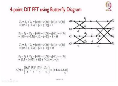
We will see the example how we will be calculating it. So, you have been given values as  $-0.5\ 2$  -0.5 and -2. So, now we will see that if we because 4 point, so we will apply the decimation in time FFT butterfly diagram is shown here. So, if we input the thing, so and then compute our  $X_0$ , so, we have worked out this example. So, if you want to see the steps have been given here, so, the first  $X_0 = 0$ , and then the  $X_1 = 1 - j4$ . So, third again is 0.
