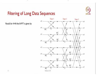
So, we know that filtering of long data sequence how we are going to use our FFT. So, as we have already discussed, we have N = 8 and 8 point FFT is given by this butterfly structure. So, you have seen the thing so, if it is 16 you can extend it and 32 and so on. So, it is easy to write N = 8 so, which we can use it.
