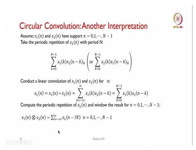
So, another interpretation is what is it? So, they have the support of 0 to N - 1. So, we are going to take the periodic repetition of  $x_2(n)$  with period N in this case, so, you will be seeing that  $x_2(n-k)_N$  and then we conduct the linear convolution instead of circular convolution, we will be doing the linear convolution of  $x_1(n)$  and  $x_2(n)$  then what happens  $x_L$  is represented as the linear convolution of n is given by  $x_1(n)$  linearly convolve with  $x_2(n)$ .
