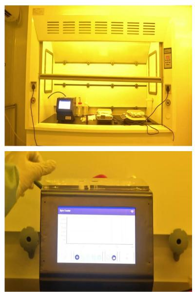
Hello, everyone. Today we are going to see how we can spin-coat polymers to obtain flexible substrate. What we are going to do is, we are going to use a precursor. It is similar to that what you have seen for a photoresist spin-coating and we will be using a carrier wafer in this case, it is silicon three-inch wafer. We will spin-coat on that, the precursor, the polymer that we want to obtain is a flexible substrate.
