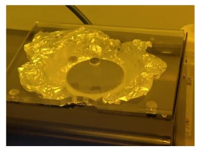
So now, we will see a hole, the precursor of the polymer can be spin coated onto a carrier silicon wafer. So, my colleague is showing how to place the silicon wafer, we need to be very careful. We will place the polish surface exposing facing us and non-polish surface, in case of single side polish silicon wafer.
