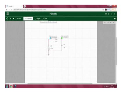
So, I will go to the grapher so here you can see since it is a simple resistive divider network and I am applying input voltage of 10 and the both the resistance of 10 both the resistances of 10k and 10k as we know that it is  $\frac{V}{2}$  so since V = 10 so output will be 5 volts and both the both the resistance are in series so the total resistance is of 20 kilo ohms so 10 volts divided by 20 kilo which is of 0.5 milliamps of current.
