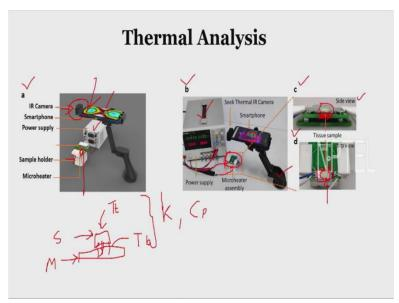
What do we have is one of the configuration that we build we have the power supply over here and we have the sample holder over here and then we have the micro heater. So, this micro heater which is placed just below the sample. So, the micro heater is like over here and then on top of it there is a sample so, this is the tissue sample and this is the microheater. This microheater actually heat the bottom part of the tissue.
