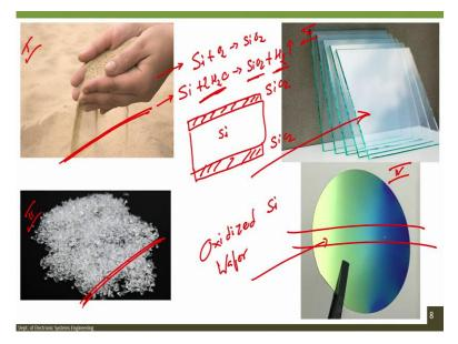
So, you can see here, the slide shows the left topmost slide shows the sand, this is a sand and through sand these are the glass crystals and this is glass right very easy to see and what is this, this is oxidized silicon, oxidized silicon wafer, oxidized silicon wafer that means you have a silicon wafer if I draw a cross section of this wafer, it will be the one that I am showing you here.
