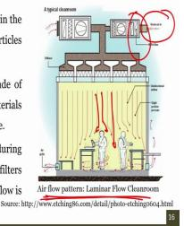
Next one is about the airflow and you can see in this particular schematic that airflow which is a laminar cleanroom flow is very important. In this case the air is introduced and recirculated in cleanroom after removing dust from the HEPA filters, you can see here the air comes from here it passes through the HEPA filters and usually the filters and docks are made out of stainless steel and to ensure minimum number of particles.
