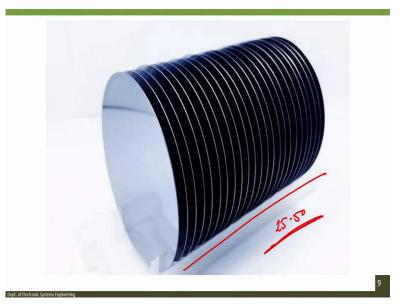
These are the racks of silicon wafer, racks of silicon, rack of a silicon wafers, all stacked together, it can vary from 25 to 50 depending on how many silicon wafers you can, you want to oxidize in one time, you can do oxidation of all the silicon wafer in one go in something called or in a process called thermal oxidation, which uses horizontal tube furnace, we will see that process.
