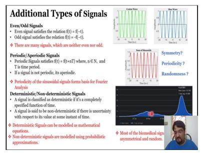
So, I hope it is clear what is even and what is odd signal, how it is look like, just remember even signals symmetrical to Y axis, odd signal symmetrical origin. So, the symmetric point is now clear I suppose you understood it properly, this is the summation of sine wave and cosine wave.
