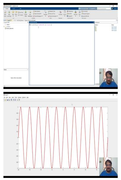
Let us see the demonstration for you, (())(5:00) signals, I have defined some variables, time variable, which is nothing but -20 to +20. Just to demonstrate the behaviour with respect to both sides of x axis, if it is symmetrical to Y axis, it is even signal, if it is symmetrical to origin it is odd signal.
