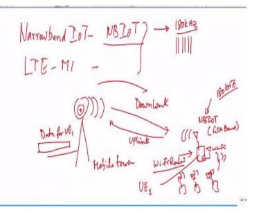
One such standard that was finalized by 3GPP organization is called the narrowband IoT. When you say narrowband IoT, this is interesting because it is really narrowband. It is using a 180 kilohertz of bandwidth; that is all. Remember what your bandwidth was in LoRa, it was 125 kilohertz. Here it is 180 kilohertz. Again, there are multiple channels here. Again, there are multiple channels.
