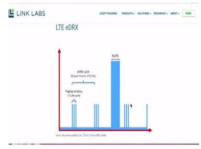
So the picture shows something interesting. Shows the power profile of LTE-M1 UE that means end device, the IoT device, which has aggregated data from several sensors, and it is we are talking about the lifetime of that device, okay. This is a picture directly showing you the eDRX mode. Now the DRX mode is go back and look folks at what you have done here folks.
