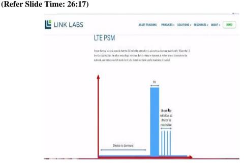
That comes out by the LTE PSM which is true also for narrowband PSM. This is even more fantastic. What does it do? Here the idea is the UE tells the network, that means the end device tells the network it is going to go dormant indefinitely. Do you not think that this is very similar to the what type of device, the Class A device of LoRaWAN, right? Nothing but Class A. It is equivalent of Class A.
