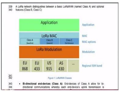
You see here LoRa modulation 868, 433, US 915 and AS 430. LoRa modulation comes in here. LoRa MAC, Class A Class B Class C we know this very well now. There are applications which you build on top, right. So it is easy now for you to pick up from here.
