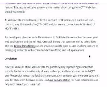
And WebSockets are built over HTTP and standard, you know the standard HTTP ports applied to IoT Hub, with the stay as 80, HTTP uses 80 instead of MQTTs 1883. And for secure connections that is 443 port number. Instead of MQTTs 8883, right. What is also interesting is what you can do with Eclipse Paho. For developers plenty of code libraries exists to facilitate connection between your web applications and IoT Hub.
