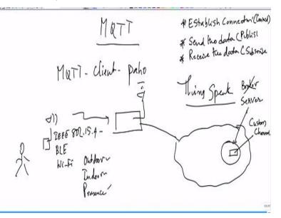
In other words, suppose you have a sensor, IoT node sensor okay, which runs MQTT client and I gave you the name, Paho. You can run on a small embedded node. You
