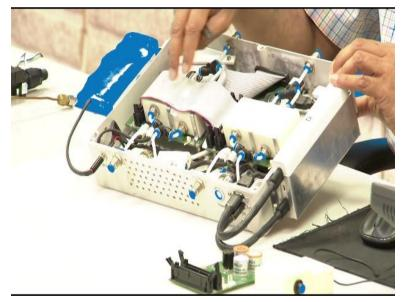
So let me draw your attention to this little box here, which has several components. Maybe I should tilt a little bit in this direction so that it will help you to look up the different components. What this has are two identical units on either side and it is doing air quality check from automobiles. One of them is taking from automobiles and the other is taking from ambient, right?
