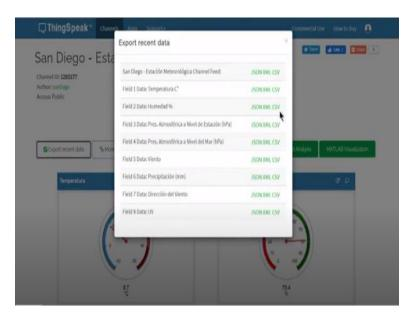
You can get it in CSV, XML, JSON, right? CSV is comma delimited file. XML and JSON are machine readable formats, which you can directly build. You can take it into another machine. You can write a program for one machine to suck this data and consume this data without humans. If you do CSV, you are stuck. You have to download, you are to open Excel or any one of these spreadsheet applications and you can plot it.
