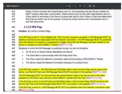
Wll says if the Will Flag is set to 1, this indicates that if the Connect request is accepted a will message must be stored on the server and associated with the network connection. The Will message must be published when the network connection is subsequently closed unless the Will message has been deleted by the server on the receipt of a disconnect packet.
