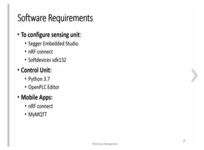
So, what did they use? They use Segger embedded studio, they use nRF connect, simple app. The soft device that they ran from nRF is SDK132. Control unit is essentially python 3.7 and also the open PLC editor which is coming from the open PLC system. So, there is a editor, you can use that. Then there are mobile apps you can either use nRF connect which comes along with the chips that you buy, the components that you buy.
