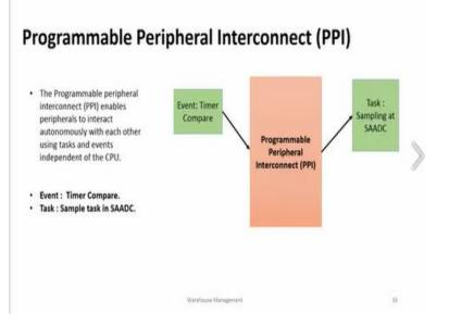
It is called PPI without disrupting the CPU, the CPU can continue to be sleeping. You can have even timers which will trigger periodically and go and acquire the data from the ADC and store the value and then go and interrupt the CPU. All of that you can do with programmable peripheral interconnect and that is shown here.
