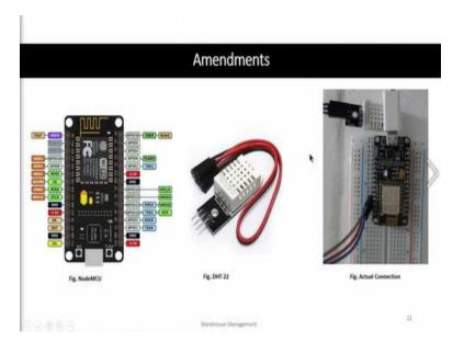
And you could also not necessary to use only those sensors and that microcontroller. You can also open up a little bit and see if you can try other type of sensors and controllers and that is what they the students actually tried. They used instead of Nordic 532 they used node MCU as their controller, they use DHT 22 as the sensor of interest and the actual connection is actually shown here.
