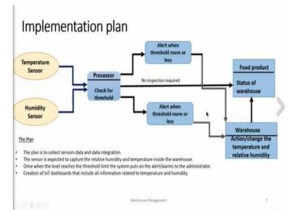
Here is the implementation plan as proposed by the students. Temperature sensor you have a system which will check for the thresholds and an alert will be issued and the status of the warehouse will be known to you. Similarly, if it is for humidity you will get at threshold. And then you may have to definitely do one thing no use in getting an alert. If temperature is going very high you must have a way to cool it down.
