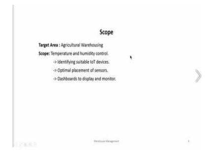
They said that let us put the scope to agriculture warehousing and temperature and humidity control are two important parameters for them. Identifying suitable IoT devices optimal placement of the sensors and dashboard to display and monitor including the personnel who is actually maintaining the warehouse should get super information about what is the current state of these two sensed parameters which is temperature and humidity control. And why are they important?
