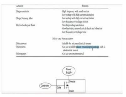
So, again, shape memory alloy is something that is very popular under this broad category of smart material based actuators, micro motors, micro valves, micro pumps all of them come under micro and nano actuators. They are all mostly PCB mounted kind of micro motors very small motors, suitable for micro mechanical systems and they can be available using silicon processing technology and it can be like a micro motor on a chip.
