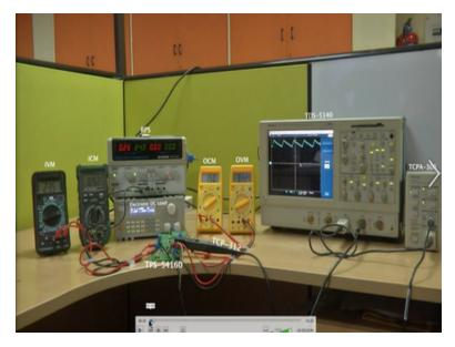
The experimental setup comprises off extreme left is the input voltage meter. The one next to that is the input current meter. Next to that are two pieces of equipment one is a power supply; this is a linear power supply. And down below is a electronic load where you can apply a certain amount of load current to the output of the buck converter and study its efficiency and performance and so on. Now, what you see on the right side?
