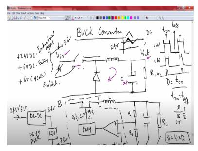
We showed that this is a simple picture of a buck converter. What do you have here? You have input voltage and you have an output voltage coming here. The input has to be higher than the output voltage. That is when you call it a buck converter and you have a transistors switch here and you have the diode for the off condition of the transistor. So, that the current continues to circulate in the circuit here. And this is the output capacitor.
