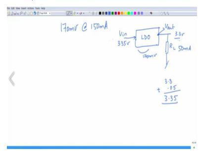
It says 170 millivolt at 150 milliamps. So, folks, this is interesting right? If my load current I will put back the LDO and output is Vout here is your input which is Vin, this Vout is let us say 3.3 volts. The load connected to this is, I have shown with the resistive load, is drawing 150 milli amperes 3.3 is the output I now add 3.3 volts plus 0.17 at the input. This will be 3.47. If I give 3.47, 170 will drop and I will get 3.3.
