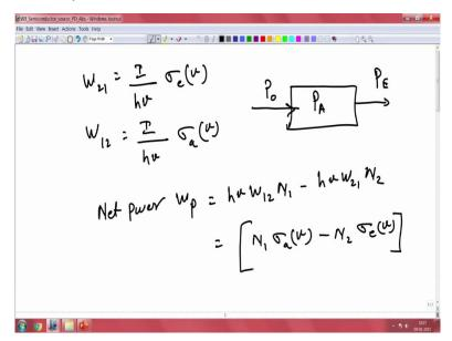
So, let us pick up from where we left in the last class. So, we had mentioned that we could write the absorption, let us say, the rates as a function of photon flux that we have for both emission and also absorption here. So, what the average power, so the average power that you have inside is nothing but the difference between the absorption in the material and the emission.
