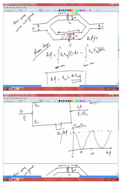
So, in a waveguide geometry we take a very simple waveguide, we put out a Y-splitter; and then we allow it to propagate through a waveguide section, and then we can combine this. So, this is basically your Mach-Zehnder interferometer using wire waveguide; so this is all single mode in configuration. In this case delta phi is 0; you can see here there is no difference between these
