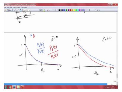
So, let us look at power coupling, qualitatively here as a function of 1, so this is 1 and this is 1 by 2 let us say and this is when delta is 0 and you start from 1 and this is 0.5, so I will pick up again A and B, so the power exchange between the counter directional coupling modes would look in a like a decay functions it is a hyperbolic here, so you start from 1 and what you will see is just the k down and the go like this and for B also you will have the same thing.
