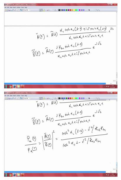
$$\begin{split} \tilde{A}(z) &= \tilde{A}(0) \left( \frac{\alpha_c \cosh \alpha_c (l-z) + i\delta \sinh \alpha_c (l-z)}{\alpha_c \cosh \alpha_c l + i\delta \sinh \alpha_c l} \right) e^{i\delta z} \\ \tilde{B}(z) &= \tilde{B}(0) \left( \frac{iK_{ba} \sinh \alpha_c (l-z)}{\alpha_c \cosh \alpha_c l + i\delta \sinh \alpha_c l} \right) e^{-i\delta z} \end{split}$$
