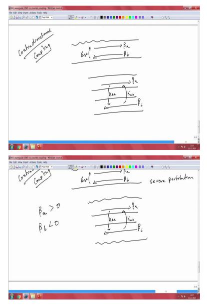
So, let us look at counter directional propagation, counter directional coupling, so here the scenario is different, let me take you back to this cartoon where we saw the waves are moving forward in a single waveguide and also in the stew waveguide system. So, in both the cases, we have waves that are parallel but they are moving in same direction, but here in counter directional or counter propagation we are going to have it in opposite direction.
