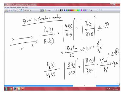
$\frac{P_A(z)}{P_A(0)} = |\frac{A(z)}{A(0)}|^2 = |\frac{\tilde{A}(z)}{\tilde{A}(0)}|^2$  $\frac{P_A(z)}{P_A(0)} = \left(\frac{K_{ab}K_{ba}}{\beta_c^2}\right) \cos^2(\beta_c z) + \left(\frac{\delta^2}{\beta_c^2}\right)$  $\frac{P_B(z)}{P_B(0)} = |\frac{B(z)}{B(0)}|^2 = |\frac{\tilde{B}(z)}{\tilde{B}(0)}|^2$
