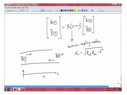
$\begin{bmatrix} \tilde{A}(z) \\ \tilde{B}(z) \end{bmatrix} = R(z; 0, l) \begin{bmatrix} A(z_0) \\ B(z_0) \end{bmatrix}$  $\alpha_c = \sqrt{K_{ab}K_{ba} - \delta^2}$
