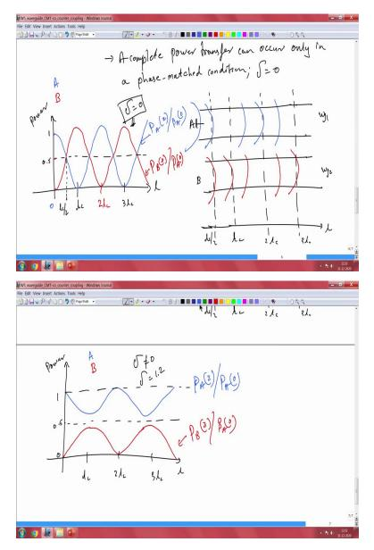
So, a complete power transfer can occur only in a phase match condition. So, what is that condition? That condition is delta should be equal to 0, so when you have 0, then you have perfect phase matching and you will get all the power coupling from one waveguide to the other, one mode to the other mode, let us look at how that will happen. So, you can numerically do that based on the equation we have, but let me show you here qualitatively how you this would happen.
