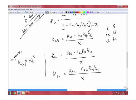
$$K_{ab} = \frac{K_{ab} - \frac{C_{ab}K_{bb}}{C_{bb}}}{X}$$
