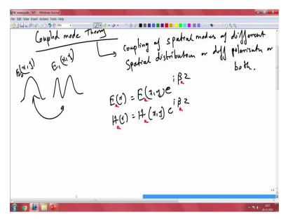
$E_a(r) = E_a(x, y)e^{-i\beta_a z}$  $H_a(r) = H_a(x, y)e^{-i\beta_a z}$
