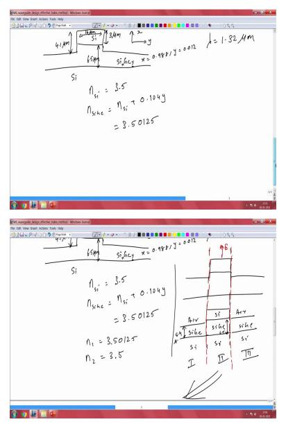
Let us see, so let us take a simple waveguide structure, let us use a rich waveguide structure. So, we have silicon substrate and I have a thin layer of silicon germanium in this case and then I havesilicon on top, this is a standard example that I that I have here. Let us do something important here, because silicon germanium can take, a refractive index based on the composition of silicon and germanium. So, let us say here, x is 0.988 and y is 0.012.
