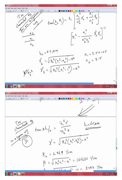
So, next let us look at TM characteristic equation, for a, for an asymmetric waveguide. So, what is asymmetric waveguide here, that is our shoulder section, air, silicon, germanium silicon. So this is asymmetric, you see, so, that is why we are going to use asymmetric relation here. So a symmetric relation, you remember that it is a little complex equation here, k1 equal to k1, n1 by n2. Let us say n1 n2 and n3.
